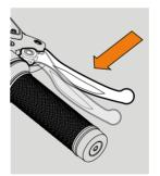
**Tip:** The brake lever angle can be adjusted to your preference using the screws on the brake lever mount. Ensure they're re-tightened to 7Nm torque setting.
